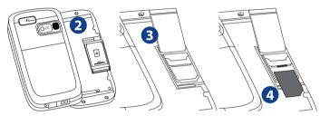
After inserting the SIM card, close the SIM card door and then lock it by sliding the lock to the right.
