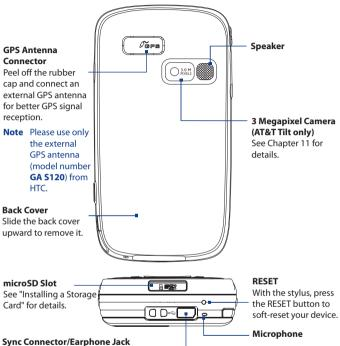
Connect the supplied USB cable to synchronize information or plug in the AC adapter to recharge the battery. You can also connect the supplied audio adapter for listening to audio media.
