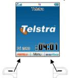
The left and right **Select Keys** are used to choose the **options** from the bottom of the screen.
