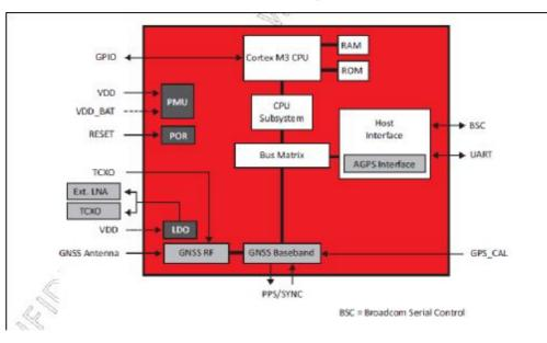
Figure 2-10 Functional blocks of the BCM47511 chip
