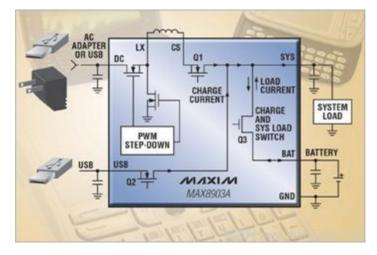
The MAX8903A can use two independent input ports or only one input port to receive power supply from a USB peripheral and an AC adapter. When external power supply is connected, the Smart Power Selector circuit allows the system to operate without any battery or operate with a battery in deep discharge mode. The Smart Power Selector circuit can automatically
