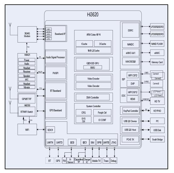
Figure 1-2 Hardware principles of the MediaPad 10 FHD
