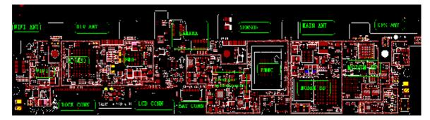
Figure 4-2 Layout of components on the PCBA
