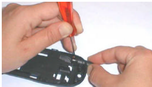
Press with a screwdriver to release the antenna
