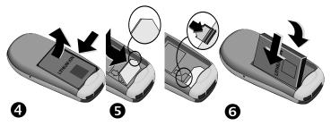
Insert SIM card in the opening, contacts pointing downwards (make sure the angled corner is in correct position §). Push gently until it engages §.
