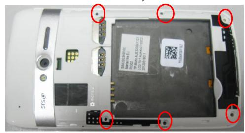
2). Remove the furnished front deco according to below instruction by using plastic flake,
