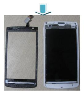
2). Please use hot wind gun to heat up LCD module around the four edges (Temperature:  $100^{\circ}$ C, Air Level: 3, Height:5-10mm, Time:<60s), and then use plastic flake to push the LCD model through the hole as below.
