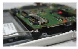
3). Remove the RF cable by using tweezers.
