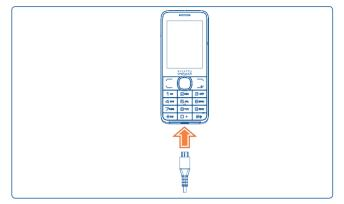
Connect battery charger to your phone and plug into the socket.
