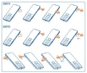
Place the SIM card with the chip facing upwards and slide it into its housing. Make sure that it is correctly inserted. To remove the card, press and slide it out.
