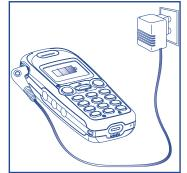
The on-screen indicator stops flashing when charging is over
