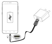
You can charge the device with a travel adapter or connecting the device to a PC via a USB Type-C cable.
