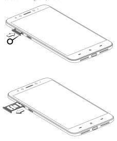
2. Insert the SIM card(s) and memory card into the tray as shown:
