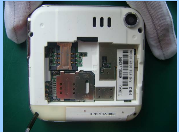
Remove 4 screws with screw driver.
