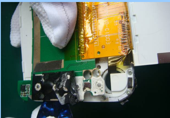
(17) separate LCD PCBA with tweezers
