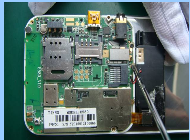
Remove 2 screws with tweezers
