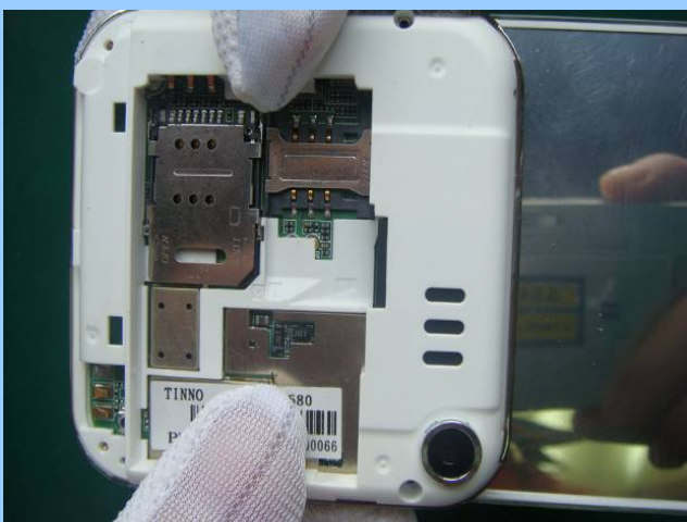
(11) Connect FPC with PCBA board
