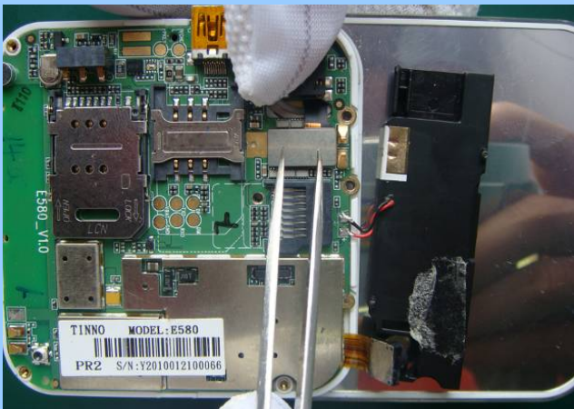
(9) Tighten the FPC connector
