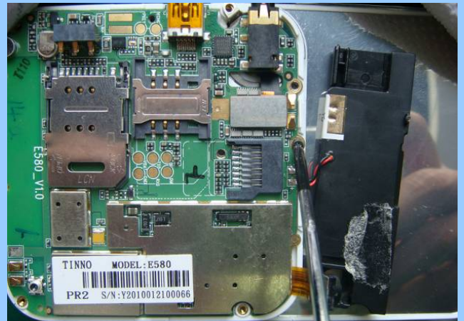
(10) Lock 3 screws with tweezer
