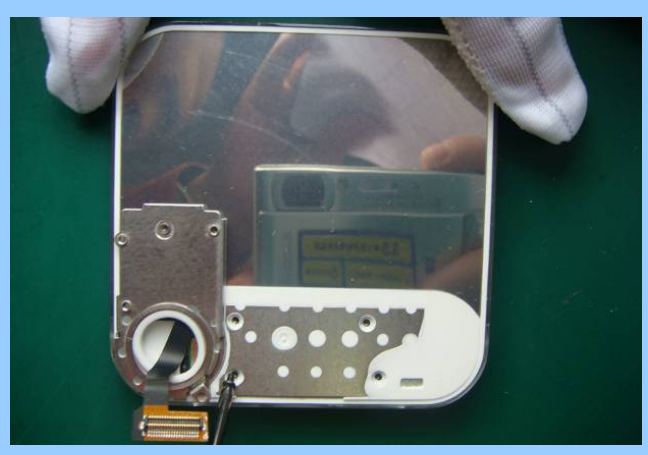
(6) Lock the screws with tweezers
