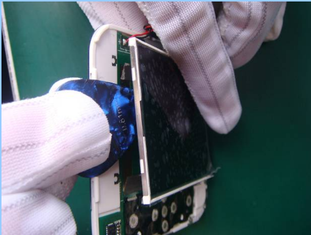
(15) Separate LCD with pick
