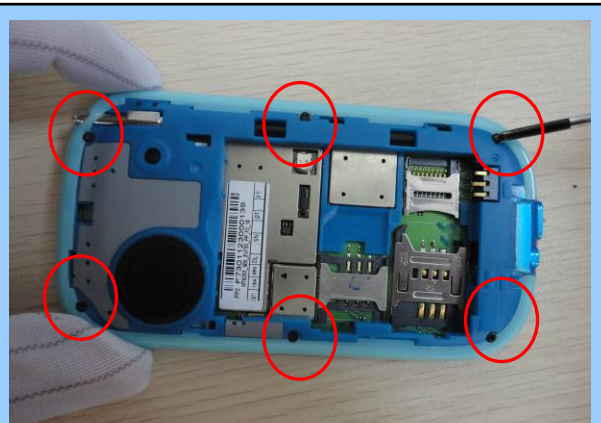
Unfasten the 6 screws by screw
