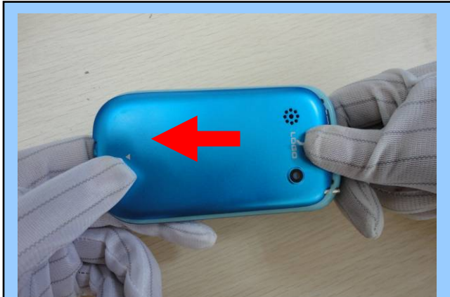
Push the battery cover from left to right
