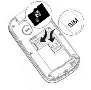
Locate the SD card holder and gently slide the card in the holder.
