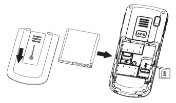
You have the option of inserting a micro SD card.
