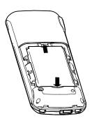
Replace the battery compartment cover back on the phone. Slide the battery compartment cover upwards until it snaps in to place.
