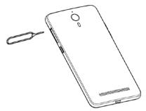
1. Insert the ejection pin into the hole to loosen the card tray.
