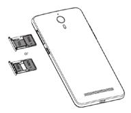
2. Pull out the card tray gently. Place the Micro SIM card on the card tray 1 and place Nano SIM card or Micro SD card on the card tray 2.
