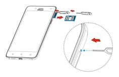
2. Put the SIM1 into the card slot on the tray
