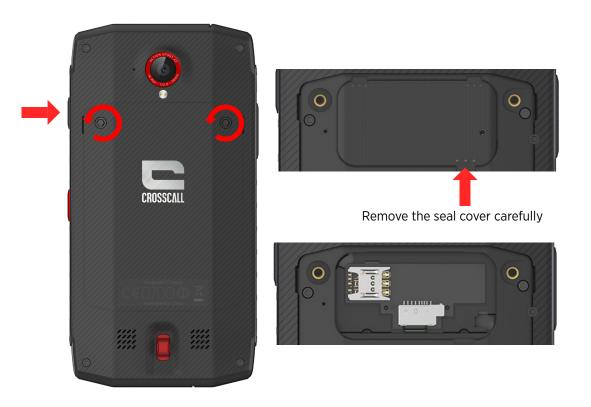
**Warning:** Take care about the antenna when you remove the seal cover. Do not use tool to remove the seal cover to not damage the rubber seal.
