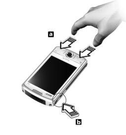
2. While holding the Today and Messaging buttons, Using the tip of your stylus, lightly press the reset button inside the hole (**b**) on the left side of your handheld.
