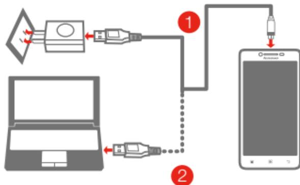
**Method 1.** Connect your smartphone to a power outlet using the cable and USB power adapter that come with your smartphone.
