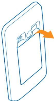
4. To remove the SIM card, pull it out from the slot.
