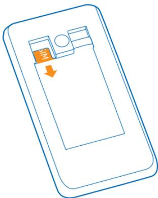
5. To remove the memory card, pull it out from the slot.
