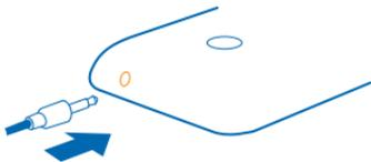
Do not connect to products that create an output signal, as this may damage the device. Do not connect any voltage source to the audio connector. If you connect an external device or headset, other than those approved for use with this device, to the audio connector, pay special attention to volume levels.
