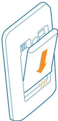
7. Press the bottom edge of the back cover against the bottom edge of your phone, and snap the cover into place.
