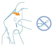
$\ensuremath{\mathbf{3.}}$  If the battery is in, lift it out from the upper right corner.
