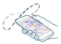
The compass has limited accuracy. Electromagnetic fields, metal objects, or other external circumstances may also affect the accuracy of the compass. The compass should always be properly calibrated.
