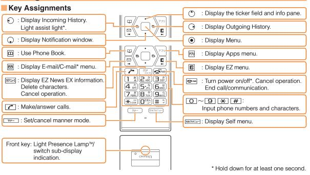
• If you lose track of where you are or if you make a mistake, press to return to the previous screen. Return to the standby screen by holding down for at least one second.
