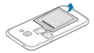
3 ► Dual SIM models: Pull out the SIM or USIM card.
