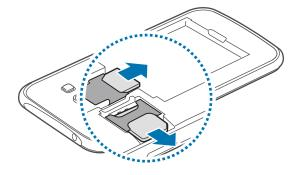
► Single SIM models: Pull out the SIM or USIM card.
