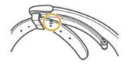
• **Metal strap:** Use the adjustment tool included in the package to adjust the strap.
