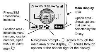
Following some operations the display will automatically clear after three seconds or after pressing any key.
