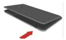
2. Locate the Micro-SIM card slot, which is on the right side (see diagram). Carefully slide the Micro-SIM into the slot in the direction indicated on the phone and in the diagram, with the contacts facing down.
